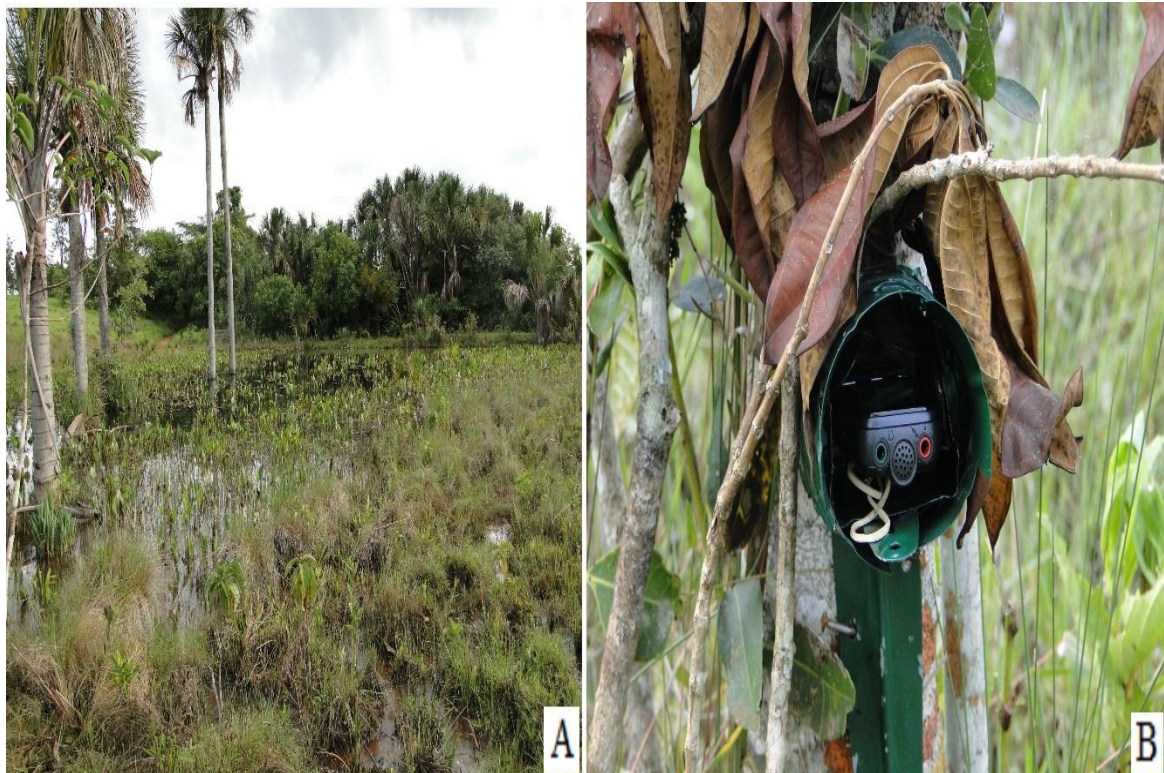
Figure 1. (A) Study site at municipality of Rio Verde, Goiás state, Brazil. (B) Adaptation of ADR using Sony ICD-PX312.
